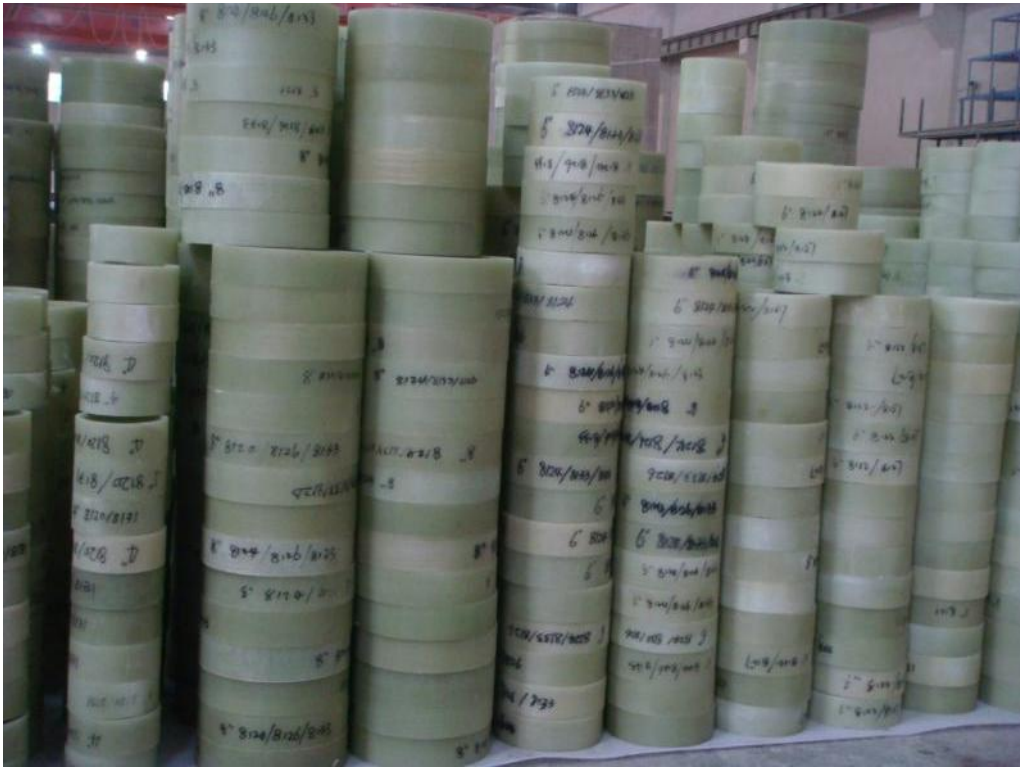
Hand Lay-up FRP Support Ring Spacers for Piping
