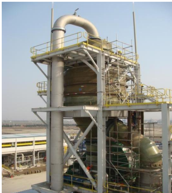
Solid FRP Crystallizer (ID.5300mmX10m H)
