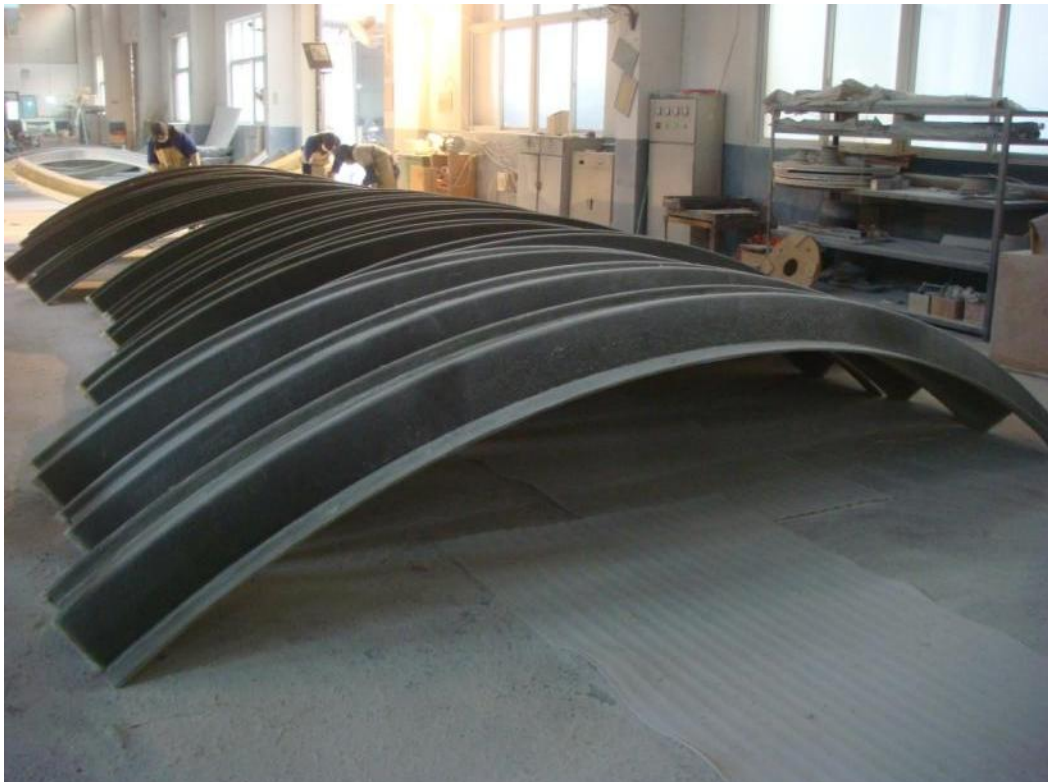
Hand Lay-up FRP Ribs
