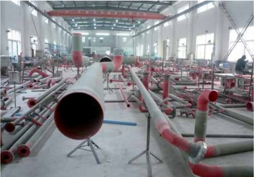
Preparation of dual laminate spools for a project in China
