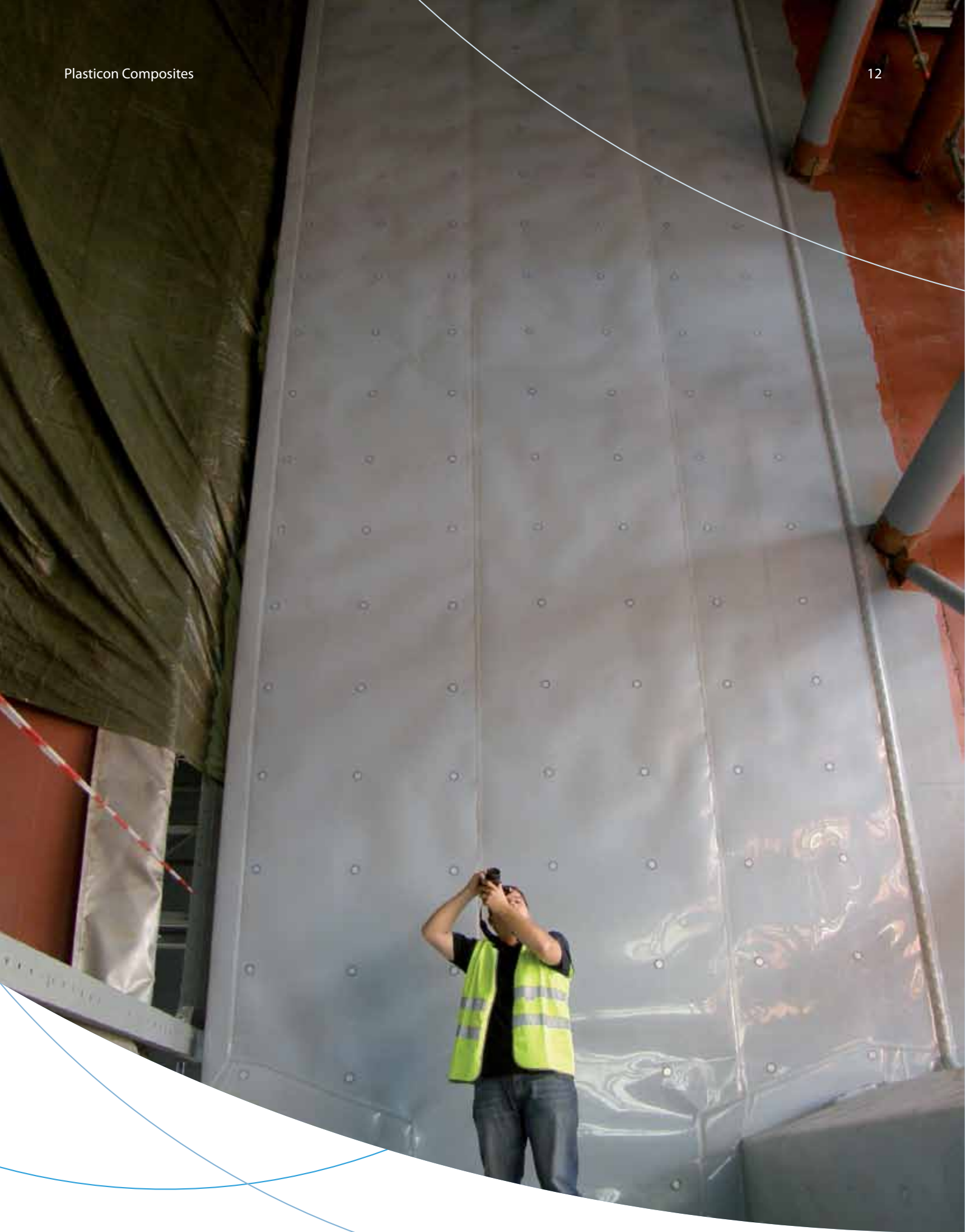
Double wall fix point lining (PFA) of a stainless steel column (D = 2000 mm)
