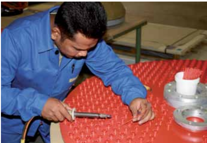
Hot gas welding of a PVC/GRP demister plate
