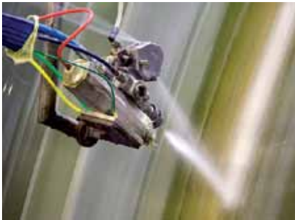
Spray winding of a GRP storage tank
